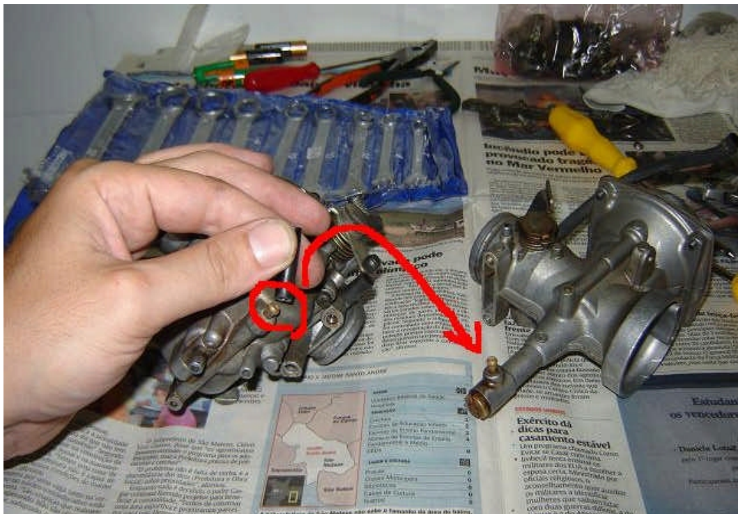
Fig 22. Remove the small hose between float chamber and the second stage at the bottom & store safely.
