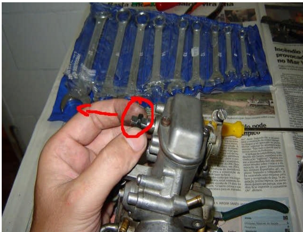
Fig 24. Slide the rubber O-Ring from the shaft.
