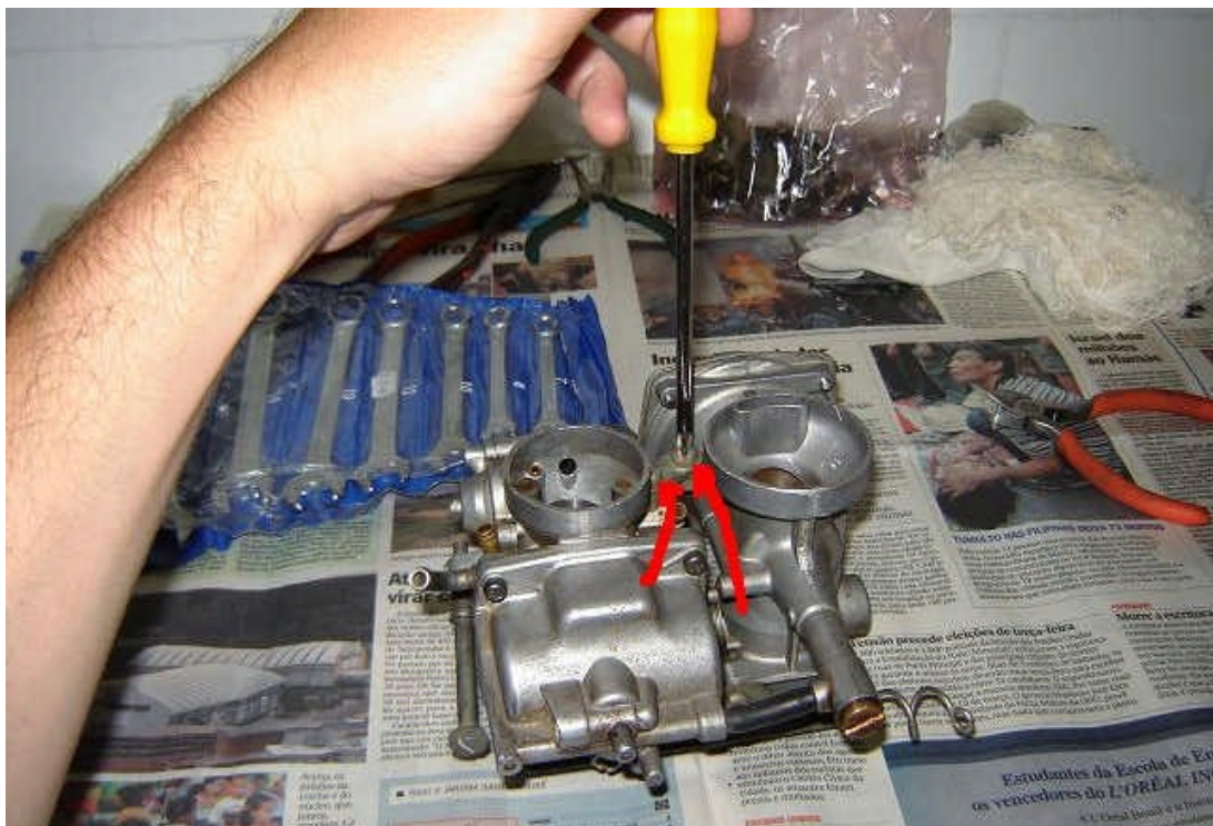
Fig 19. Remove the screws that hold the two sides of the carbs together.
