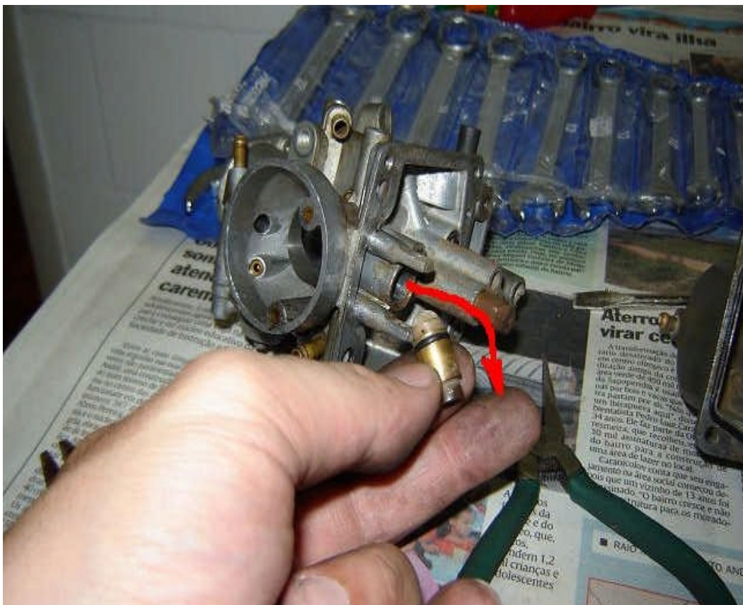
Fig 37. When you remove it you will see the filter, it is common to find it dirty.
