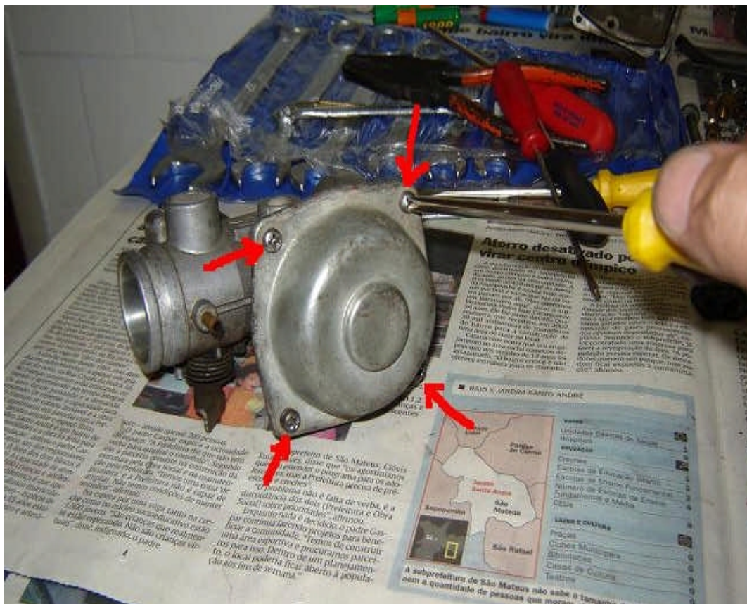
Fig 49. Remove the four screws on the diaphragm cover, there is a big spring underneath the cover so watch it doesnt go flying accross the room.
