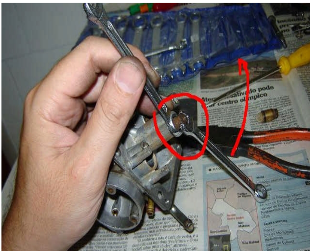
Fig 39. Unscrew the main jet, you will need two spanners (8mm & 6mm) if im not mistaken.
