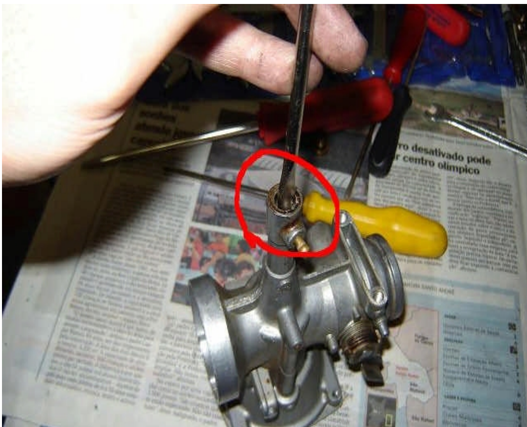
Fig 57. Then with a screwdriver undo the main jet.
