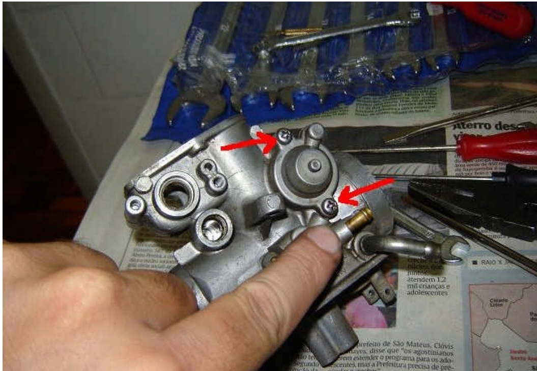
Fig 44. Remove the screws on the decompressor cover, this stops your bike popping on decelaration.
