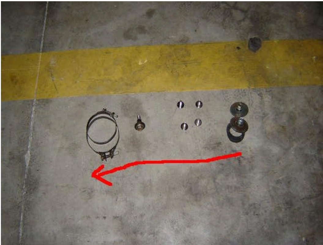
Fig 4. (Tip) Keep the parts in sequence of disassembly, this will help you remember the order when it comes to putting it back together.
