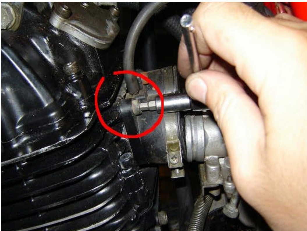
Fig 15. With the carburetor loose, we must also remove one of the intake manifolds to facilitate the exit of the carburetor out of the bike, begin by loosening the top screw.
