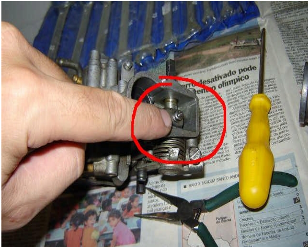
Fig 26. Once the cover is removed, undo this screw which will allow the cam to slide out.
