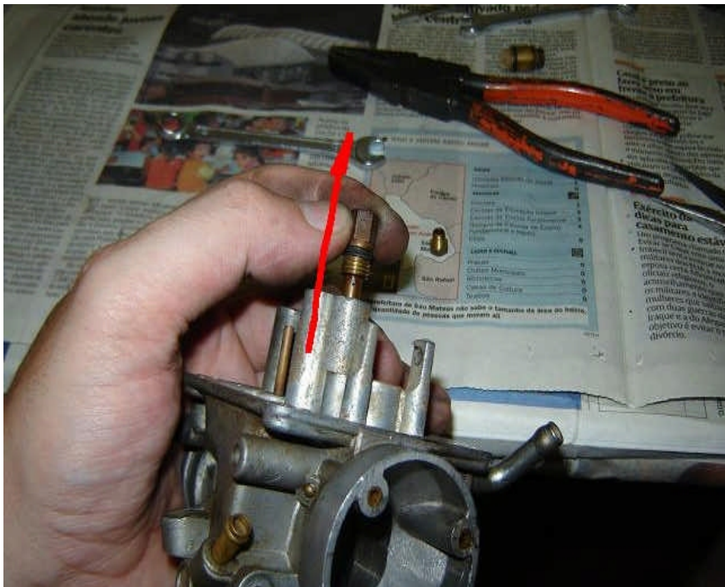
Fig 40. Unscrew & remove jet checking for any dirt that may causing a blockage, replacement parts ( 43F-14341-00-00 ) ( 360-24512-00-00 ) ( 288-14343-65-00 )
