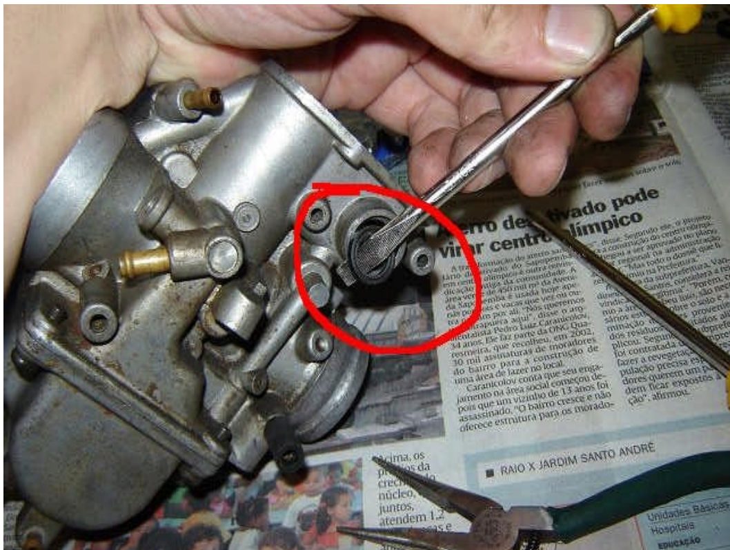
Fig 28. Remove the O-Ring being carefull not to damage it.
