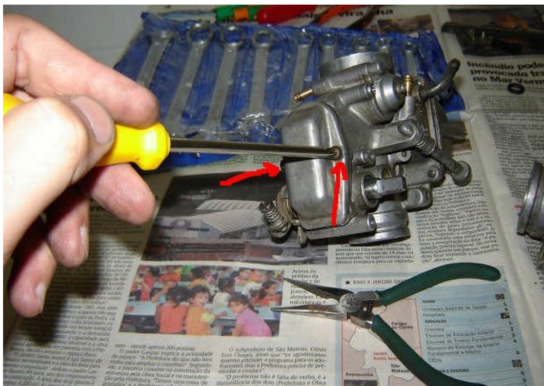
Fig 25. Remove the two screws on the first stage cover.
