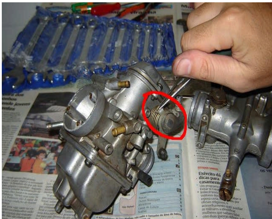
Fig 23. With needle nose pliers release the spring on the first stage carb.
