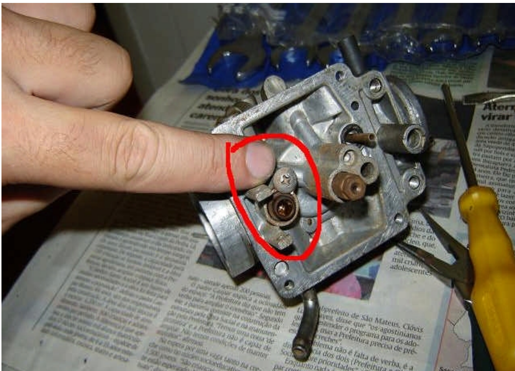
Fig 35. Remove the screw that hold the float needle seat in place.
