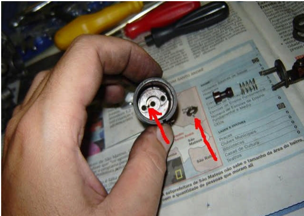
Fig 48. This hole must line up with the washer marked with arrows. when you reassemble it.
