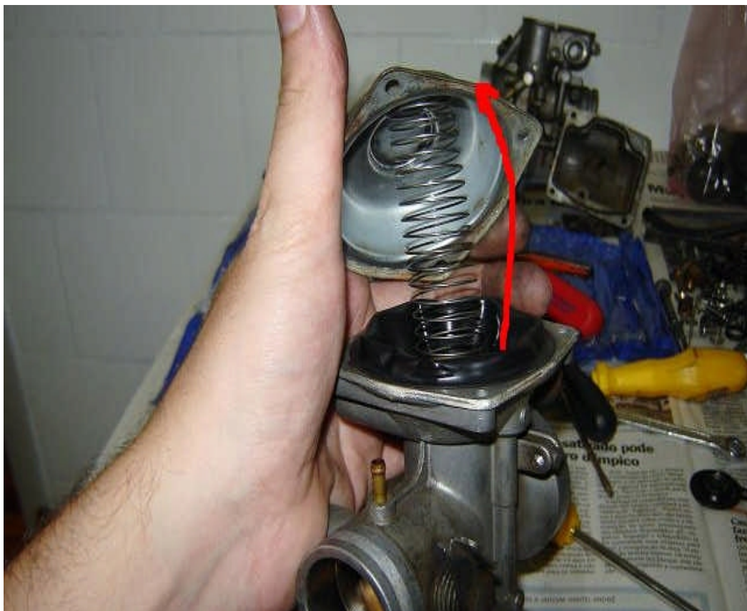
Fig 50. Remove the cover & be carefull not to puncture the rubber diaphram.
