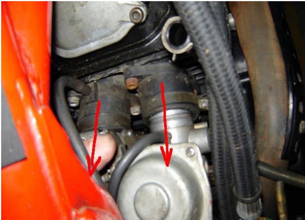
Fig 14. Gently pull back on the carbies wiggling up & down at the same time, dont go yanking on them as you will split the rubber intake manifolds.
