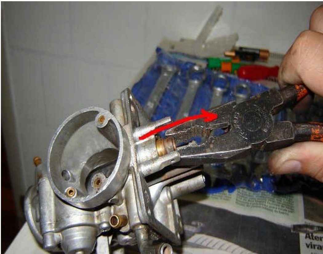
Fig 36. Pull the needle seat out gently, it can be quite tough to get out, important to remove this as there is a filter behind.
