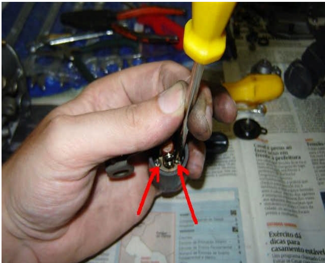
Fig 46. Remove the two screws in the throttle slide.
