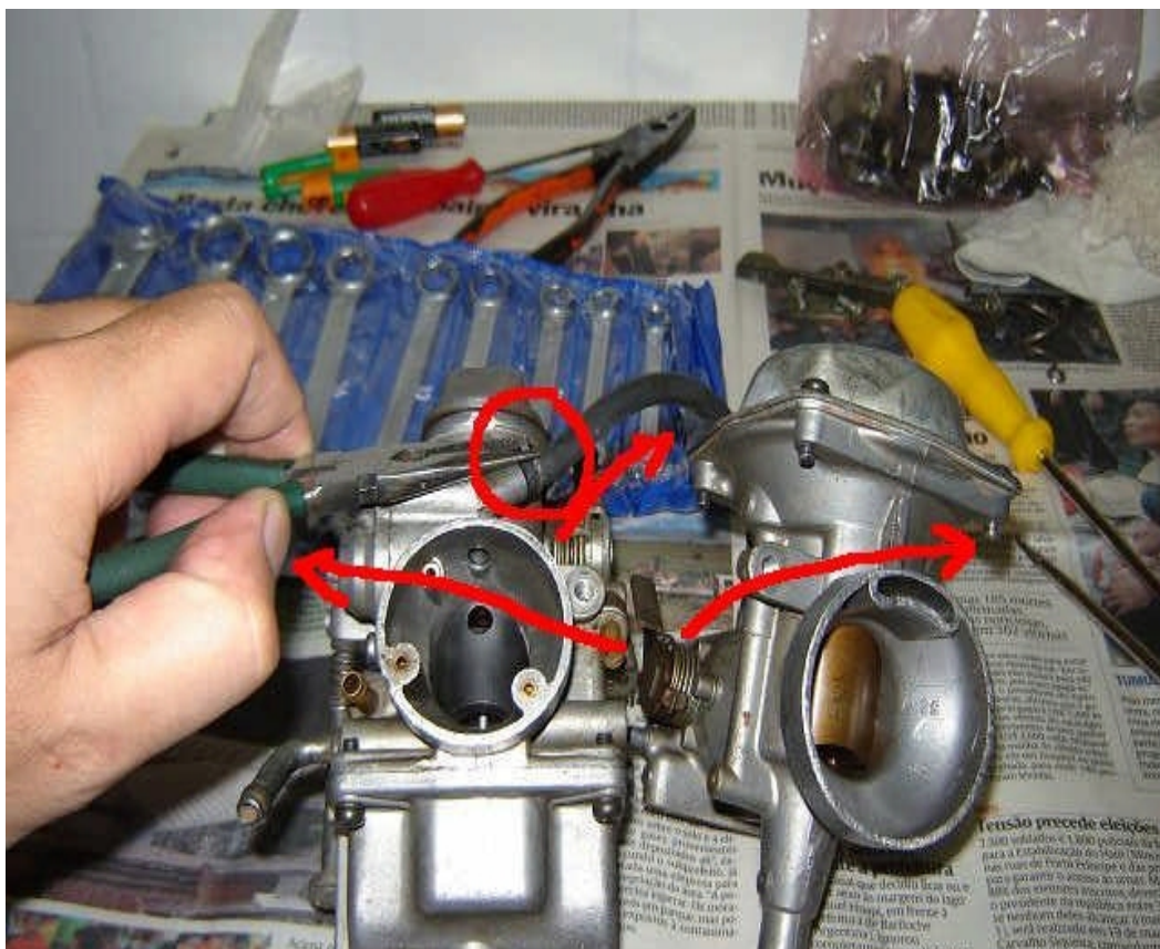
Fig 21. Release the vacuum hose & pull both sides in opposite directions.
