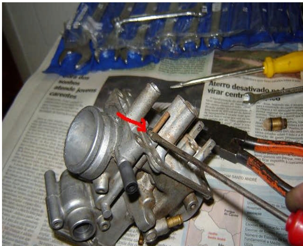
Fig 41. Remove this O-Ring carefully & keep safe or replace ( 5Y1-14536-00-00 )
