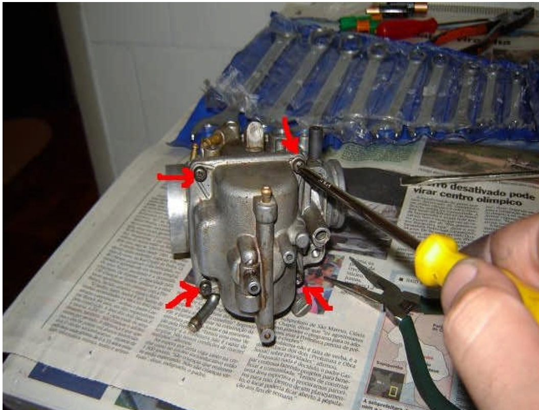
Fig 30. Remove the four screws holding the float bowl on.
