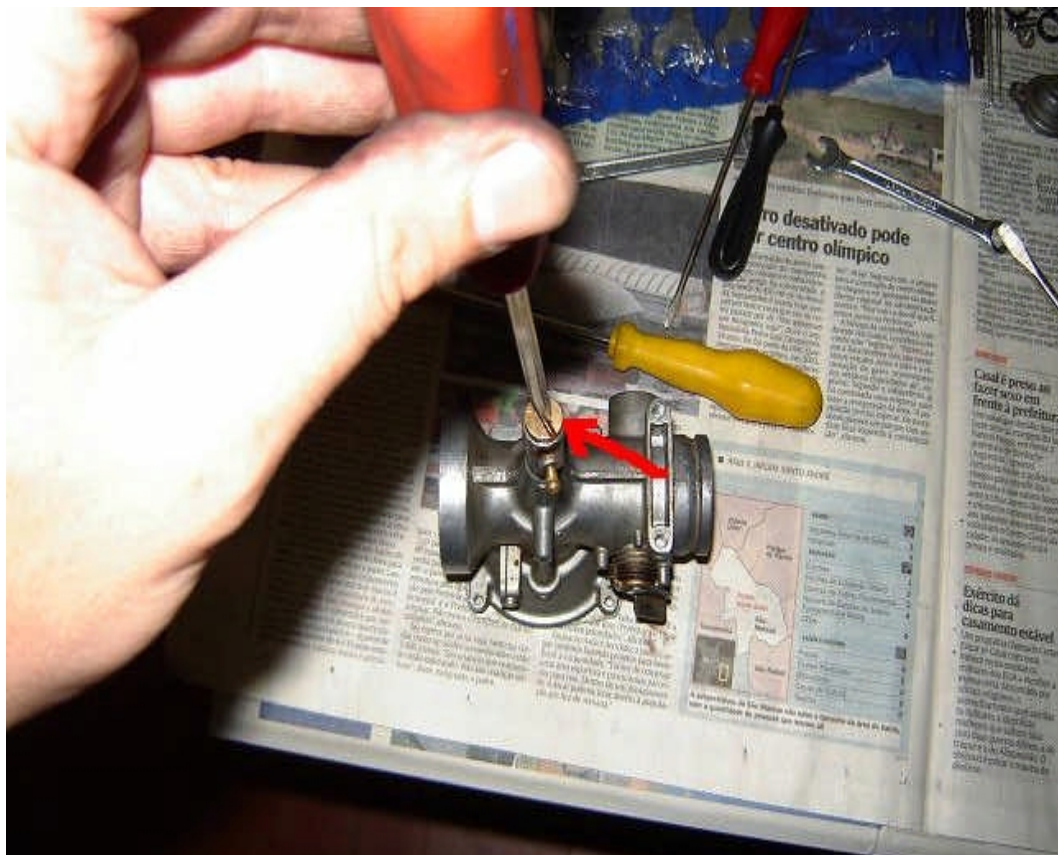
Fig 55. Unscrew the main jet ( 5Y1-14343-63-00 ) and main nozzle ( 5Y1-14355-00-00 )
