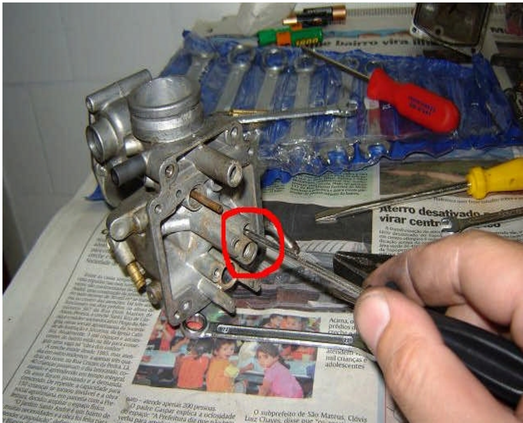
Fig 42. Unscrew the pilot jet and clean it or replace ( 43F-14342-23-00 )
