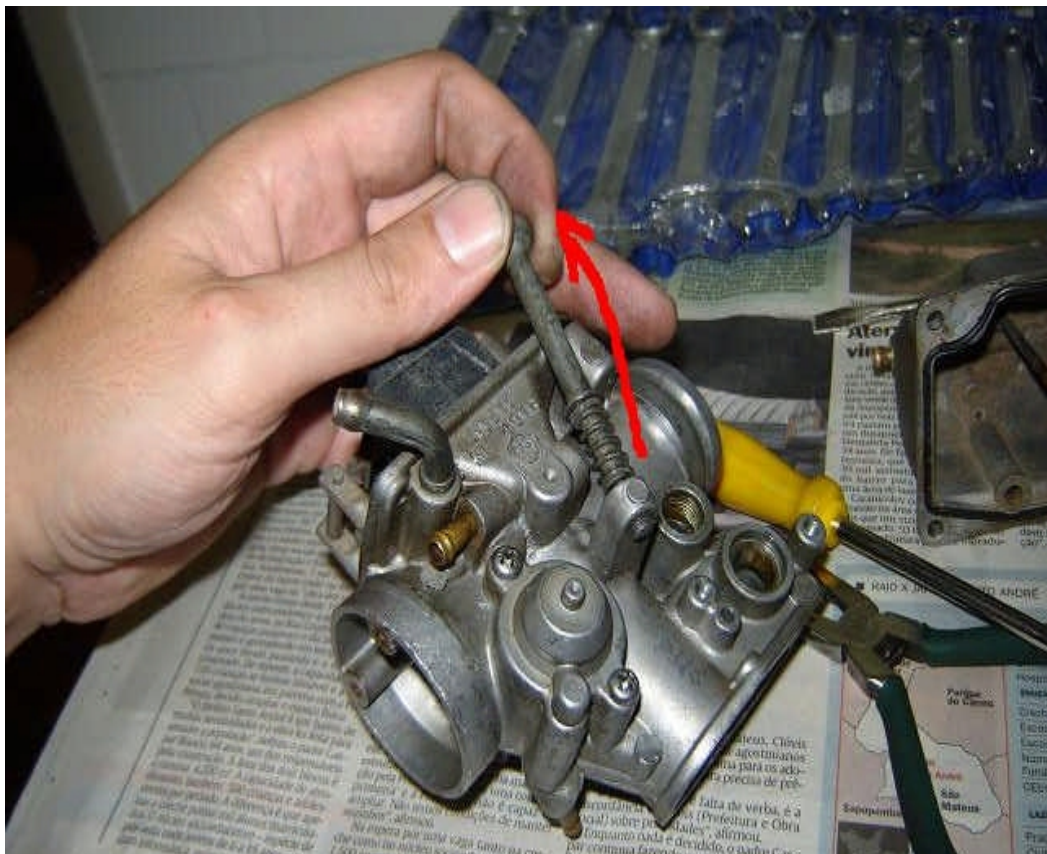
Fig 32. Remove the idle crew adjustment & clean thourogley with a wire brush, then grease & re-assemble later it, will make turing it much more easy.
