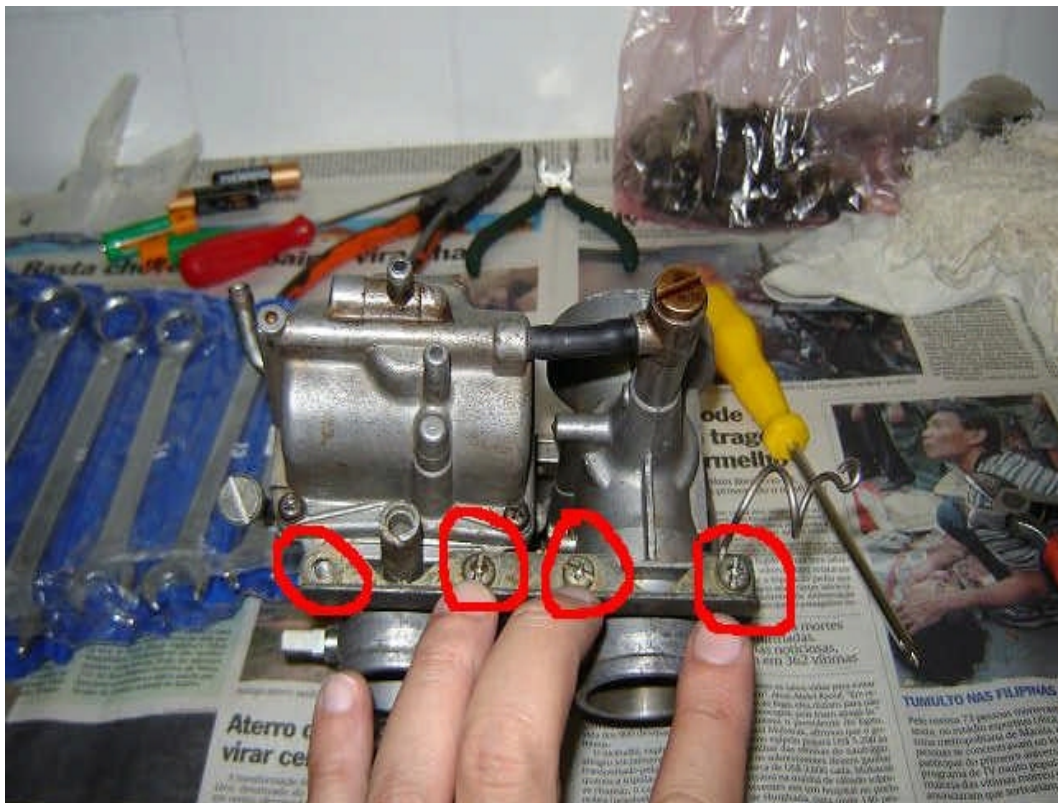
Fig 20. Then remove the four screws that hold the plate, this plate also holds both sides of the carbs together.
