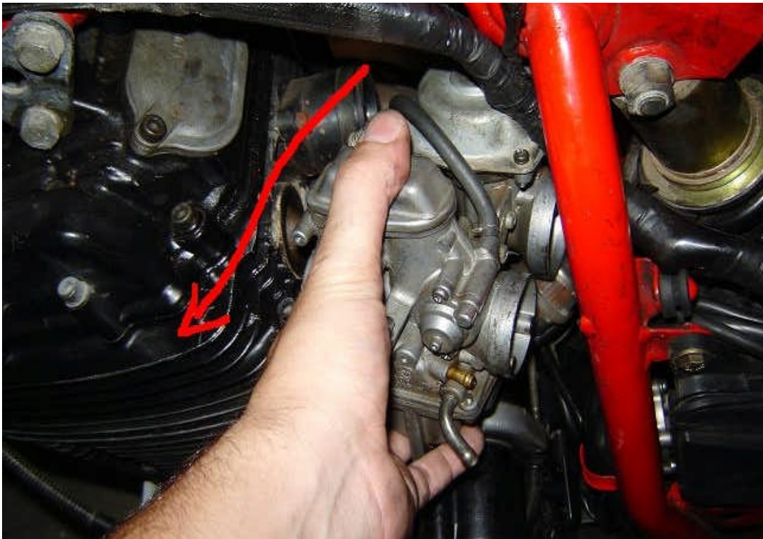
Fig 18. Then gently ease the carb out of the bike.
