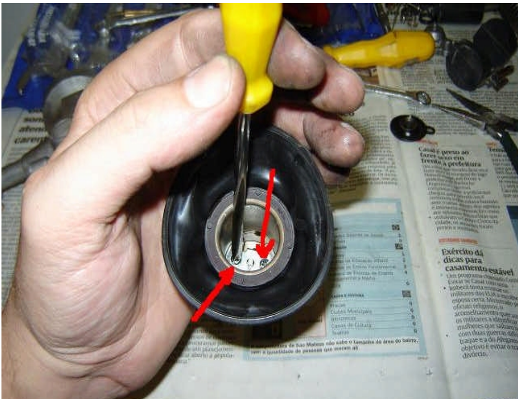
Fig 53. Remove the two screws that hold the diaphragm to the metal plate.
