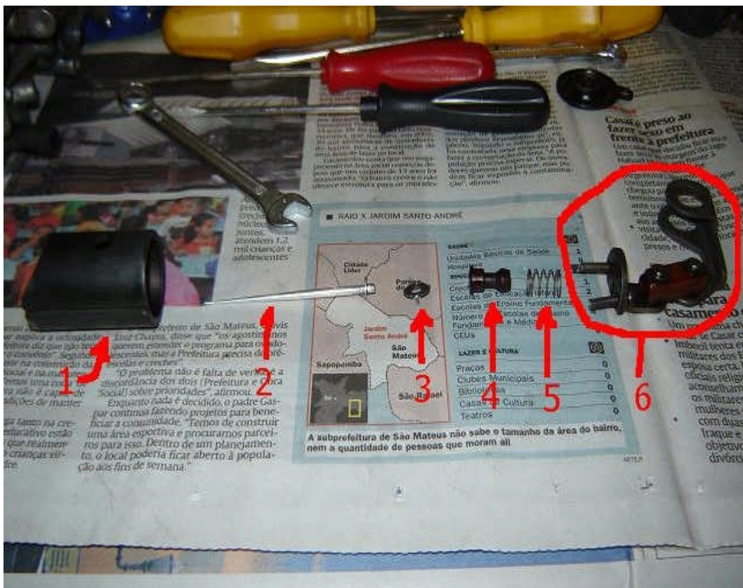
Fig 47. Throttle slide (1) Needle (2) Washer (3) Plastic connector (4) Spring (5) Cable connect set (6)
