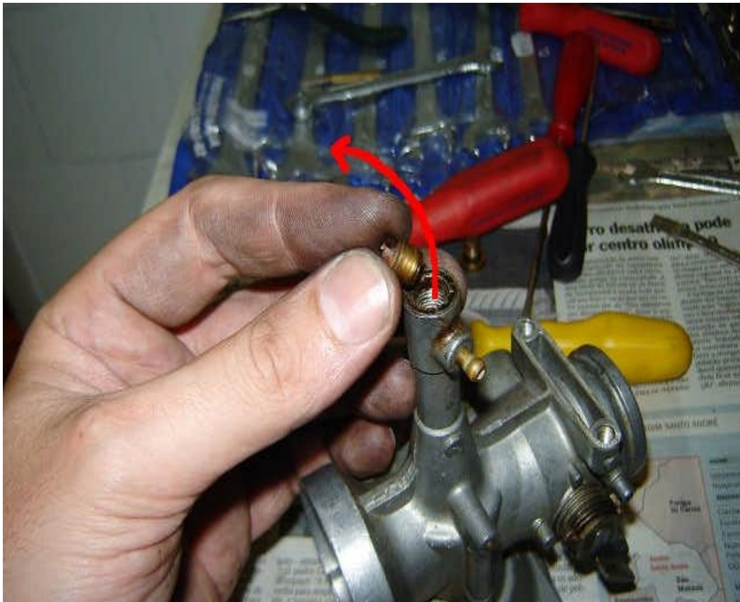
Fig 58. Taking another screw that you have access to the second needle jet I do not have a photo of this jet withdrawal but it is very simple. stick your finger in the venturi and press down to remove it.
