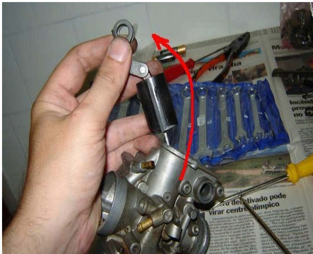
Fig 29. Pull the slide out carefully ensuring you do not bend the fine needle.
