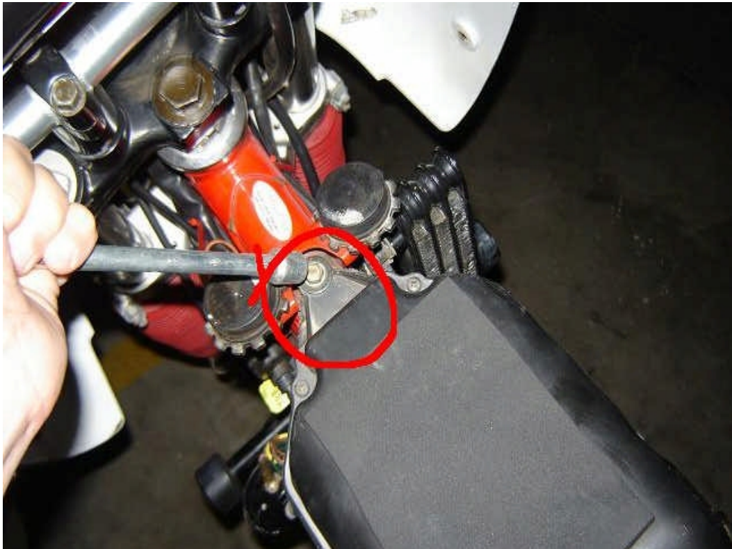
Fig 1. Remove the bolt (10 mm) that secures the air filter to the frame
