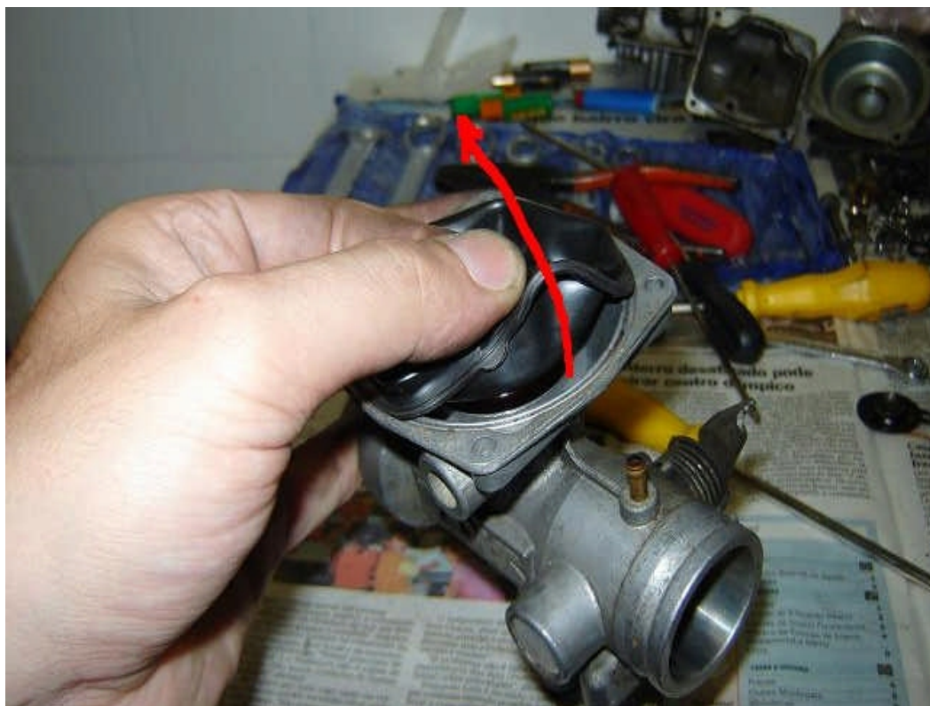
Fig 51. Pull the rubber diaphram out of the groove in the carb body, note the index mark on the rubber aligns with an indent on the carb body.
